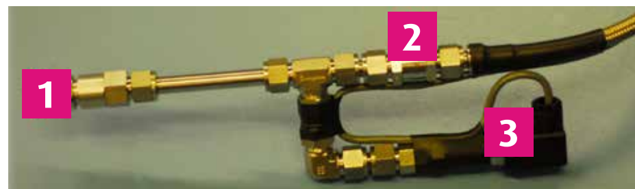
Outlet hose with sensor and non-return valve
